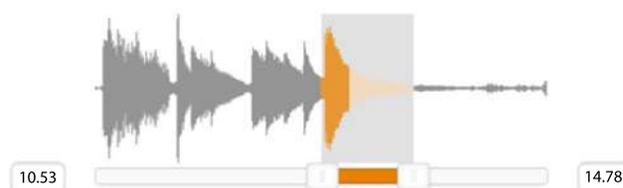
FIG. 7. (Color online) Graphical representation of the strumming sequence with the adjustable start and end markers of the loop. The same image of the waveform was used for all stimuli.
